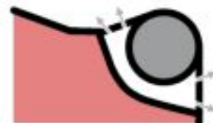
Double gasket between fluids
